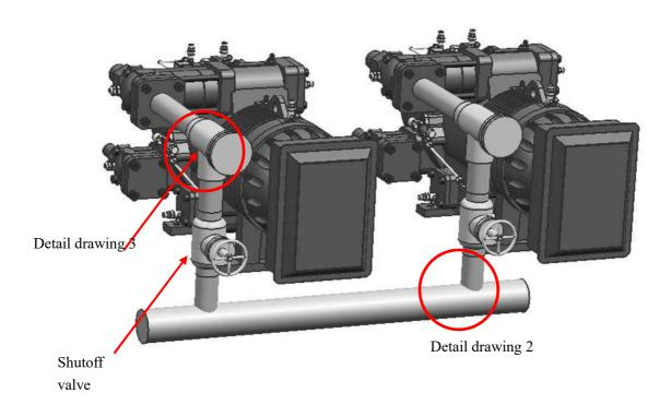
Figure 10 Suction piping diagram-parallel system
