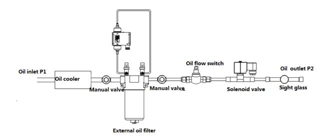
Figure 11 External oil circuit system
