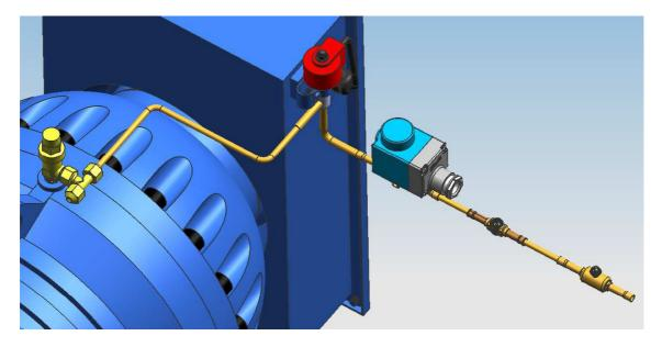
Figure 5 Electronic expansion valve installation diagram
