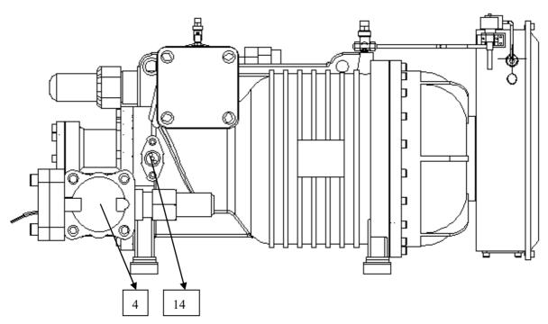
LB360/410-PLUS Low temperature screw compressor external structure
