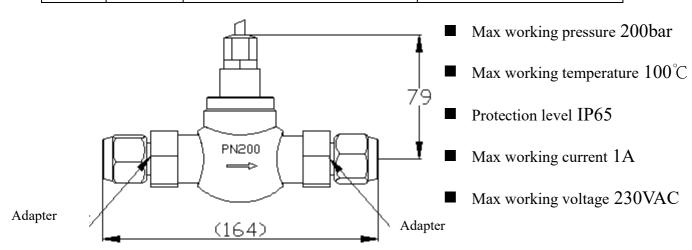
Figure 31 Oil flow switch diagram
