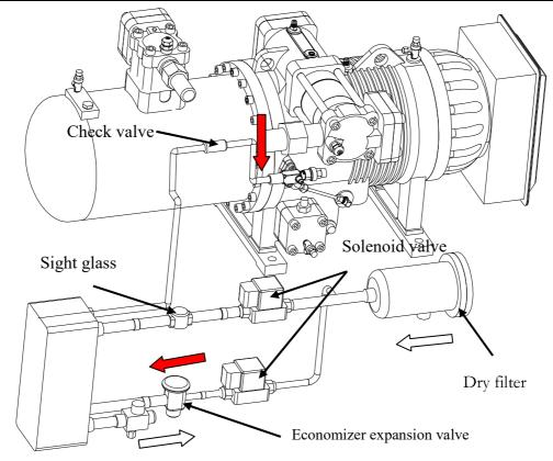
Figure 19 Economizer piping drawing - Single type
