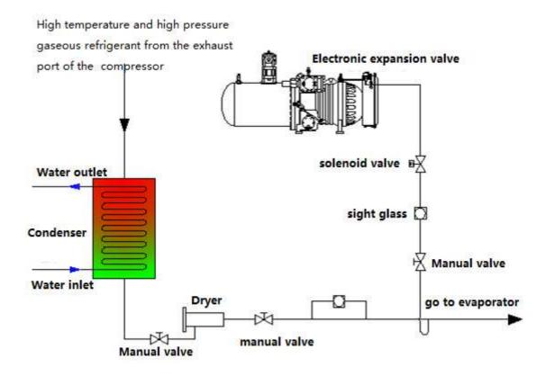
Figure 4 Motor cooling electronic expansion valve piping
