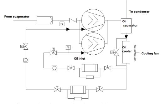
Figure 13 Air cooling type oil cooling parallel connection system
