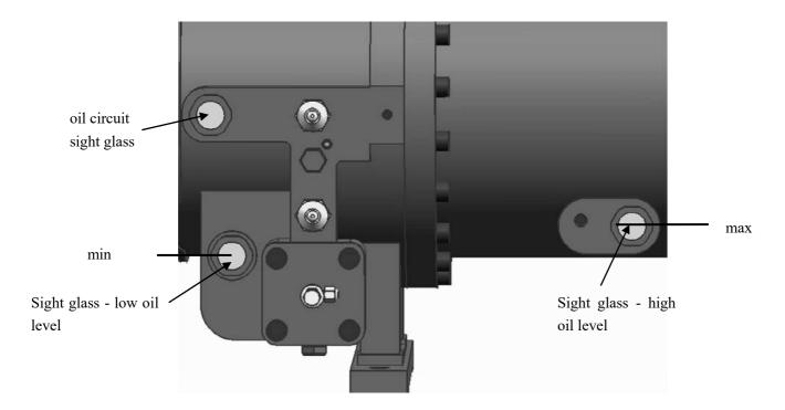
Figure 39 Compressor oil level mark
