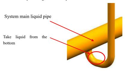
Figure 6 Liquid taken from the bottom
