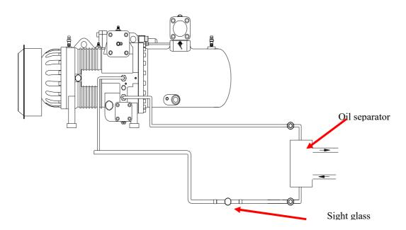
Figure 16 LB-100~280-PLUS Piping drawing of external oil cooling type oil circuit-single type
