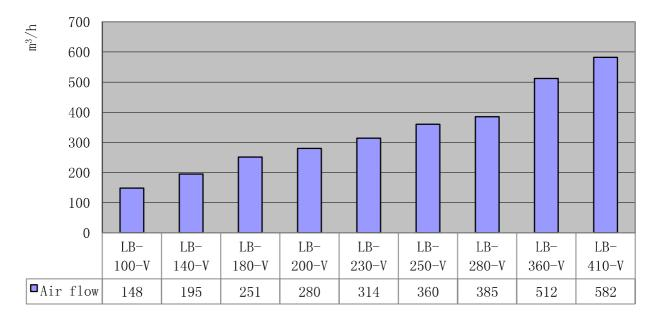
Figure 1 LB-PLUS Compressor Air Flow Specification Table
