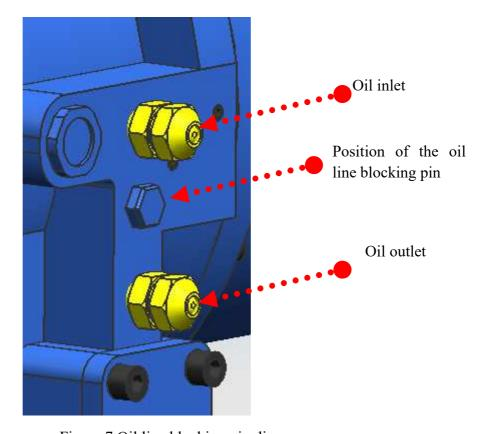
Figure 7 Oil line blocking pin diagram
