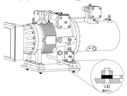
Figure 29 Installation diagram of compressor damping pad
