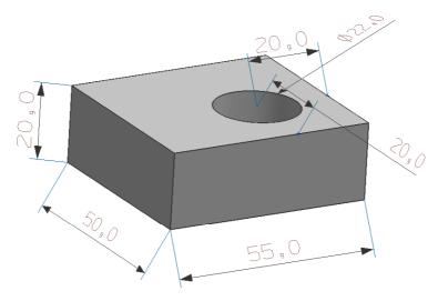
Figure 36 Compressor damping pad specification (mm)
