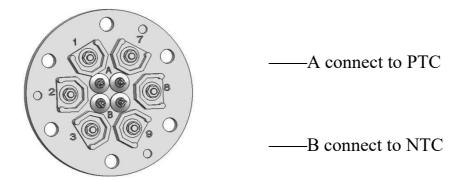
Figure 21 Compressor wiring
