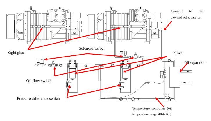
Figure 18 LB360/410-PLUS Piping drawing external oil circuit parallel connection
