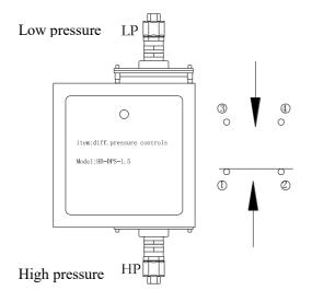
when the pressure differential switch controller is in normal state, 1 and 2 is connected; when the pressure difference increases and exceeds the set value, 3 and 4 is connected; when the pressure difference decreases and lower than the set valve, please push the reset button, thus 1 and 2 is connected
