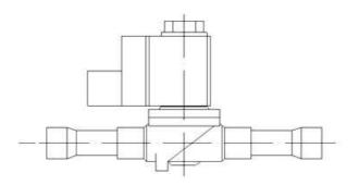
Figure 33 Oil circuit solenoid valve diagram
