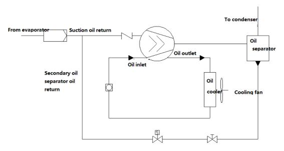
Figure 12 Air cooling type oil cooler single system
