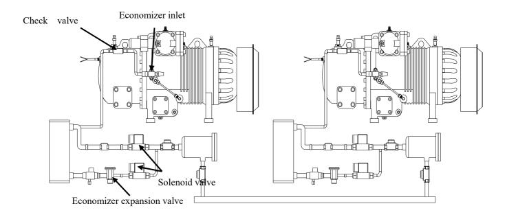
Figure 20 Economizer piping drawing - parallel connection
