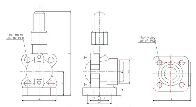
Figure 35 Shutoff valve dimension
