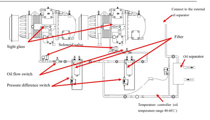
Figure 17 LB-100~280-PLUS Piping drawing of external oil cooling type oil circuit
