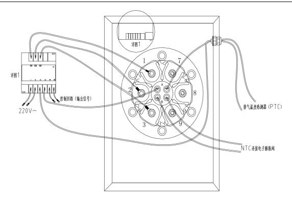
Figure 38 INT69 HBY&PTC connection diagram
