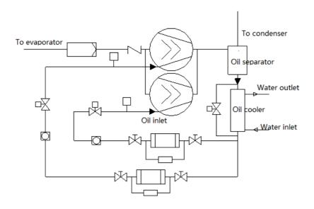
Figure 15 Water cooling type oil cooling parallel connection system
