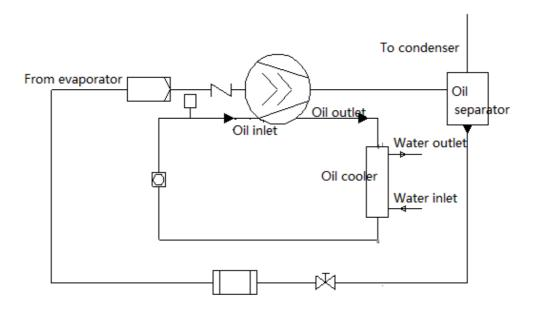
Figure 14 Water cooling type oil cooling single system
