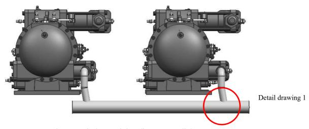
Figure 9 Discharge piping diagram-parallel system
